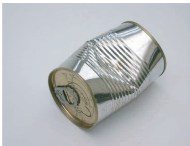
Figure 1. Typical can deformation after impact.
