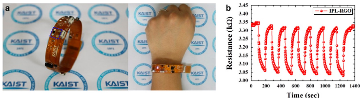
Figure 18. (a) Photograph of a wearable sensor module (wrist) integrated with the intense pulsed light-reduced graphene oxide (IPL-RGO) sensor (denoted by blue dotted box). (b) Dynamic resistance change of the IPL-RGO-based wearable sensor module to 20 ppm of H 2 S gas at room temperature. [Reprinted with permission from Professor I.-D. Kim from Korea Advanced Institute of Science and Technology (KAIST), ref 227. Copyright Springer Nature.]
